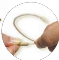
Gently pull ear hook from the headband about 1/8" to unlock. Turn ear hook into upright position. Release to lock into place.
