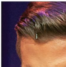
When camouflaging, the lavalier should be positioned as close as possible to the sound source for best performance. Secure the lavalier so it remains stationary without being subject to clothing noise or gusts of air or dust. Always ensure the mic is pointed toward the user's mouth.
